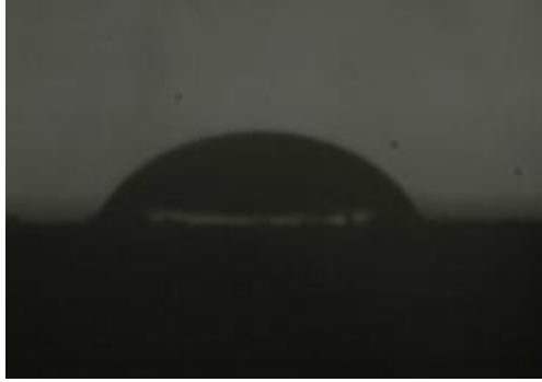
Figure 4-9: Goniometer image of a droplet of oil applied to a site.
