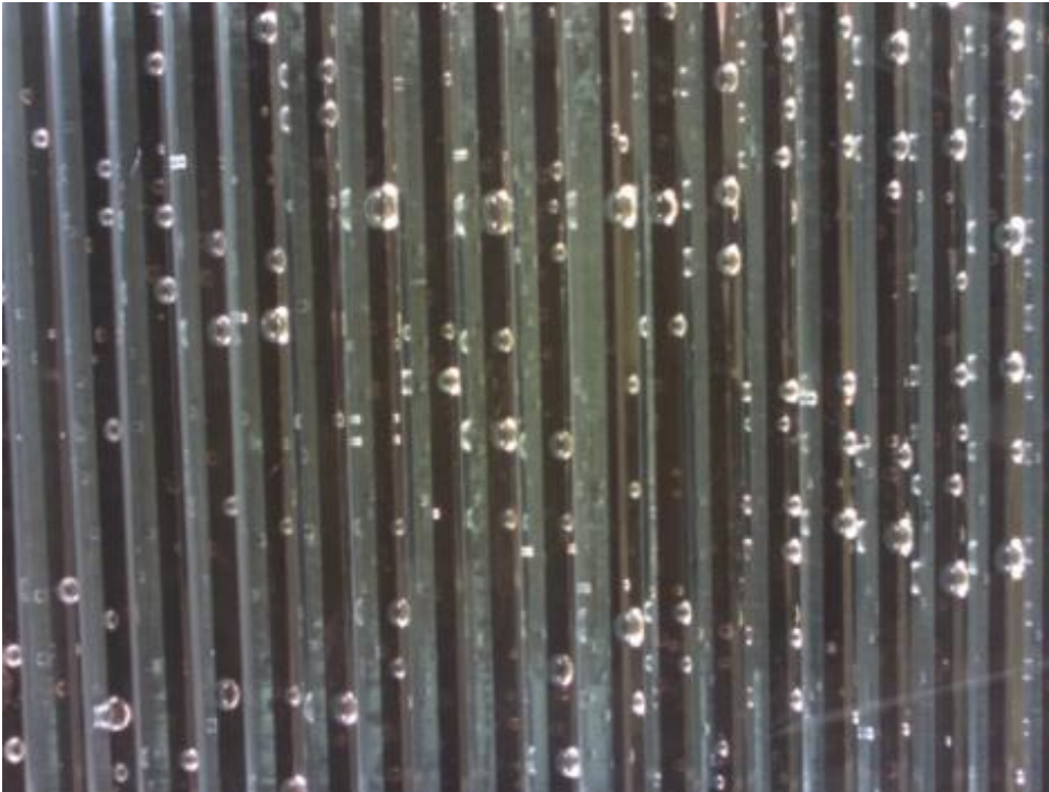
Figure 5-2: Assembly sites with bubbles.
